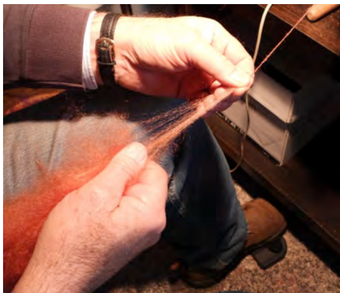
Figure 5 Draw back with the rear hand to give a uniform amount of mohair then slide the front fingers back. Don't let the twist get past your front fingers
